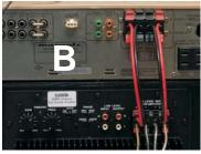
or Home Theatre Amps, simply connect the "Sub Woofer Out" RCA to either the Left or Right (or both) "Low-Input" Sockets on the XLS800 (S200W Amplifier). Power up and adjust.
