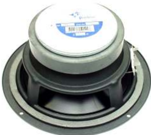
Peerless 850122 Vented Box, Vb = 30 l F3 = 032 Hz Fb = 034 Hz Response peak = 000 dB Qs = 20 Ql = 50 Qts = 100
