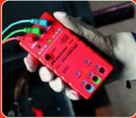
**EPMB** Safe and simple go-no-go testing for phase sequence and motor rotation, see page 16
