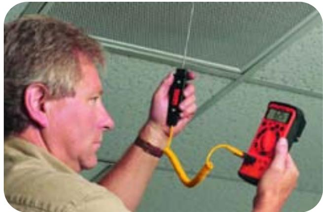
**Measures temperature. Type K thermocouple included with the 35XP.**
