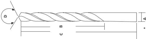
• A for size • B for flute length • C for total length • D for degree
