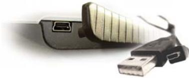
The USB socket is located under the rubber moulding on the left side on the instrument.
