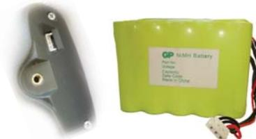
Attach the socket of the new battery to the connector on the instrument. Put the battery pack in place and put back the lid and screw.
