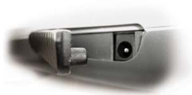
The charging socket is located under the rubber moulding on the right side of the instrument.
