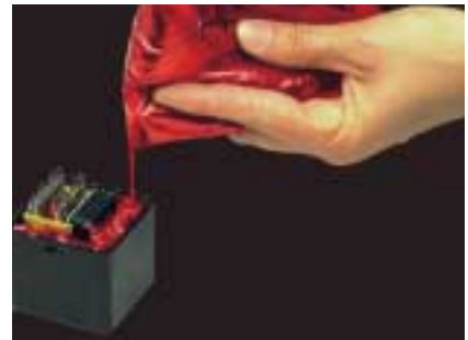
Mixing and dispensing is easy using the Electrolube resin twinpack system
