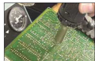
Through hole rework with the DSV80
