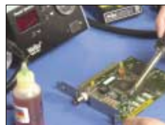
The HAP1 desoldering a component.
