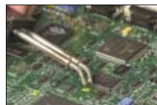
The WTA50 is perfect for removing Mel's from a SMT board.
