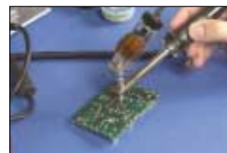
DS80 desoldering pencil with external solder collection chamber
