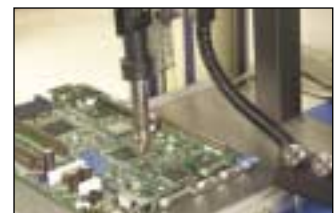
Step 3: The component is lifted off the board using the built-in vacuum pick-up.
