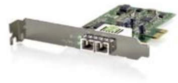
GNC-0111 1000BASE-SX Fiber Optic PCI Express Card (SC)
